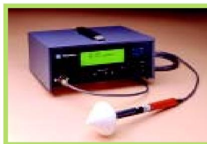
The RS-232 serial interface allows easy adapting of the unit to electronic data acquisition in laboratory studies and semi-automatic production test systems. Digital Peak-Hold and Push Button Zeroing aid in improving testing productivity and reducing errors.
