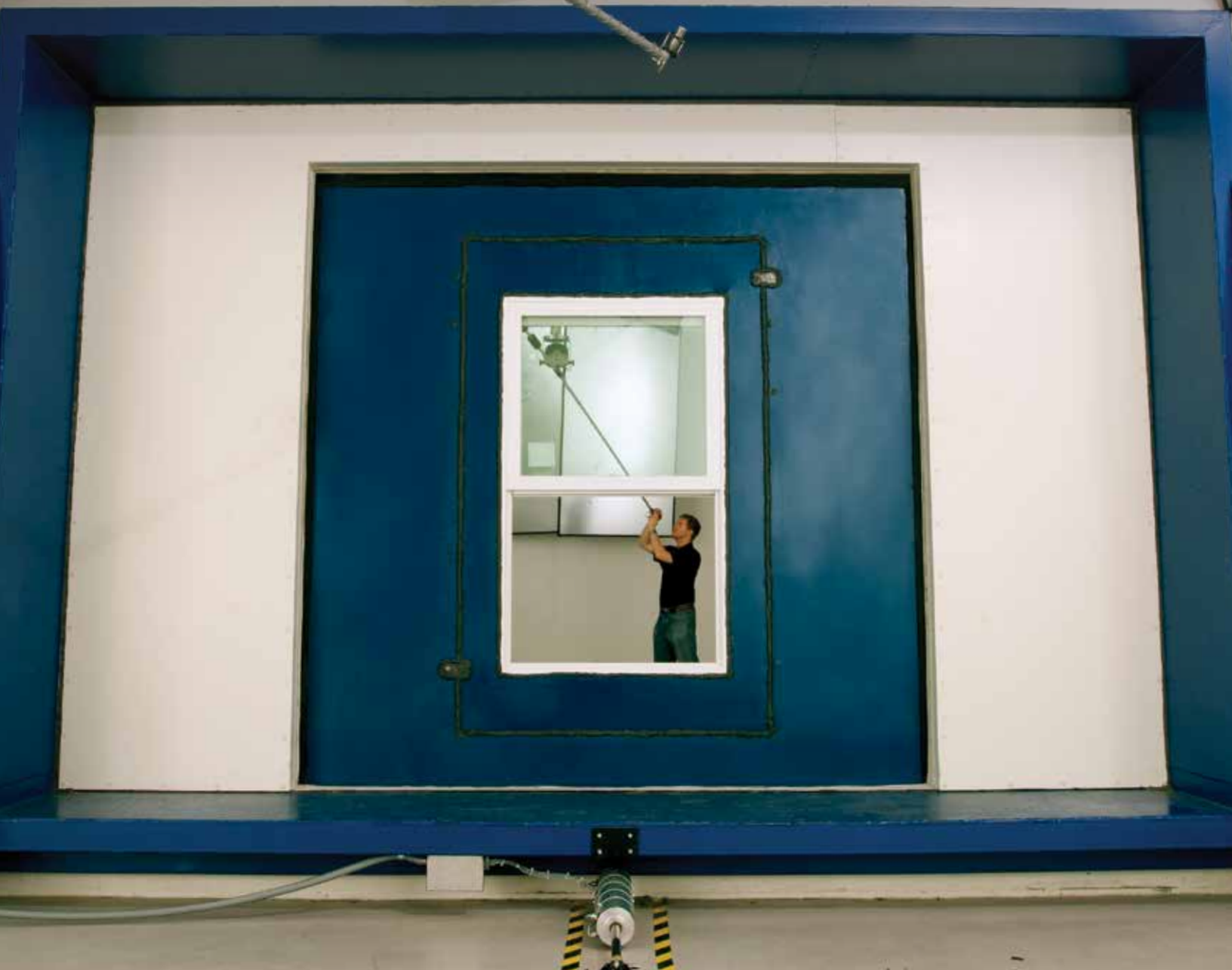
A Fenestration Test Being Performed in an ETS-Lindgren Reverberation Chamber
