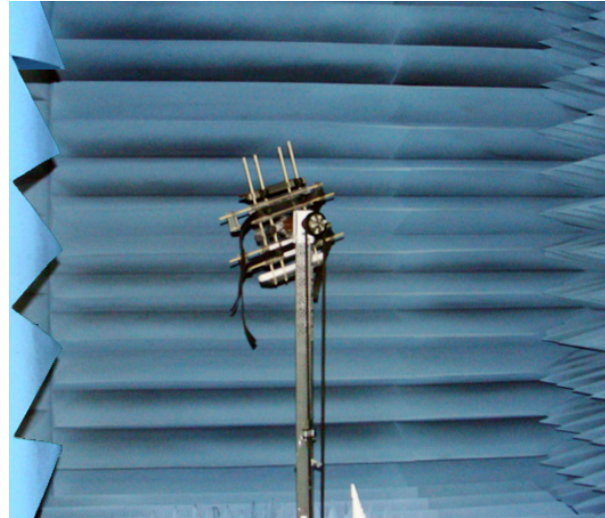
Interior of an AMS-8500 Wireless Test and Measurement Chamber
